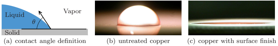
Figure 4.7: Influence of a surface finish on the contact angle.
